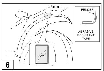
Cut in half the anti-abrasive tape and aplly to the front fender as marked, 25mm from the front bumper bar. Ensure you wrap the abrasive tape strip down around the lower edge of the fender onto the inside.
