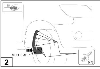
Remove the mud flaps by removing and retaining the (7) scrivets from inside the wheel arch as shown. NOTE: Replacement scrivets are supplied, if any scrivets are damaged upon removing from the vehicle.
