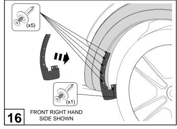
Fit the Mud Flaps to the Fender Flare and secure each Mud Flap with six (6) Scrivets supplied as shown.
