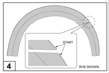
Remove approximately 50mm of the protective liner from the extrusion. Fit the extrusion to the Fender Flare along the edge that comes in contact with the vehicle's body panel. **NOTE:** Start applying the extrusion from area shown above.
