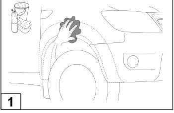
Wash the areas of contact on the vehicle and wipe dry both the vehicle and the Fender Flares with a clean cloth. Ensure inside of Fender Flares where extrusion is attached is clean.
