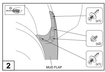
Remove the rear mud flaps by removing and retaining the (2) screws and (2) scrivets from inside the wheel arch as shown.
