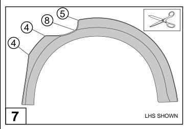
Cut a multiple triangles out of the extrusion where it meets the sharp corners as shown on the rear right flare. Note: Numbers of cut-outs indicated in circles.
