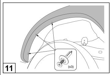
Attach the front part of the rear fender flare with 3 scrivets as shown
