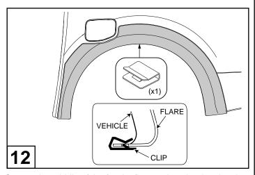
Secure the middle of the fender flare to the wheel arch using 1 small metal clip as shown.
