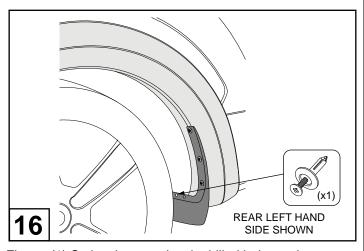
Fit one (1) Scrivet into previously drilled hole as shown.
