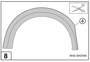
Cut a multiple triangles out of the extrusion where it meets the sharp corners as shown pn the rear left flare. Note: Numbers of cut-outs indicated in circles.
