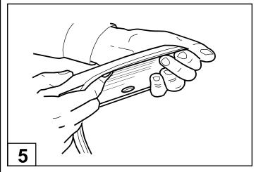
Remove approximately 50mm of the protective liner from the extrusion. Fit the extrusion to the Fender Flare along the edge that comes in contact with the vehicle's body panel.
