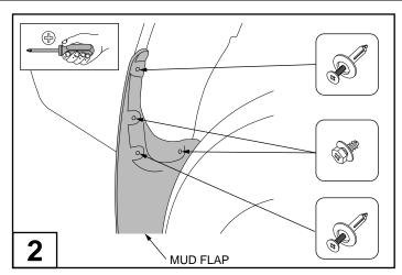
Remove the rear mud flaps by removing and retaining the 2 screws and two scrivets from inside the wheel arch as shown.
