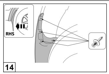
Reattach the mud flap to the fender flare using 4 scrivets as shown.
