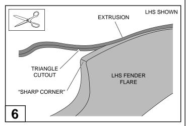
To fit the extrusion around the petrol cap cutout on the LHS flare, cut a triangle out of the extrusion where it meets the "sharp corner" as shown (fuel cap area).
