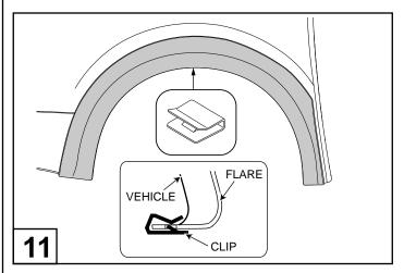
Secure the middle of the fender flare to the wheel arch using 1 small metal clip as shown.
