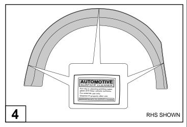
Clean the inside edge of each fender flare where the rubber extrusion will adhere.
