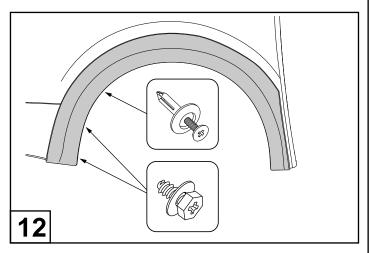
Secure the rear of the fender flare to the wheel arch using 1 scrivet and 2 screws as shown.
