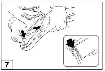
Pulling at right angles to the extrusion, remove the liner from the extrusion in small portions and apply thumb pressure to ensure that it adheres to the Fender Flares.
