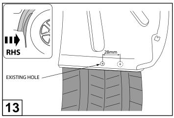
From the back of the wheel arch mark new hole 28mm outboard from the existing hole, drill with 7mm drill as shown.
