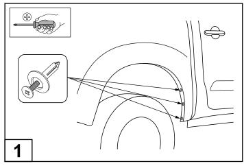
Remove the 3 screws from inside the rear wheel arch as shown.
