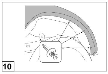
Attach the front part of the rear fender flare with 3 scrivets as shown.
