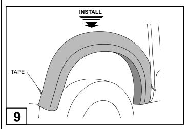
Peel back red tape liner, about 50mm from each corner of the adhesive tape on the back of the fender flare. Fit the flare to the vehicle as shown.
