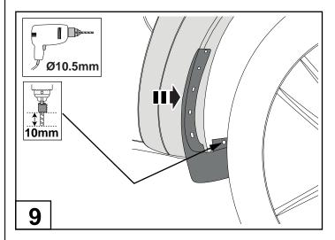
Fit the Mud Flap to the Fender Flare aligning with all the holes. Mark and drill a 10.5mm hole in the liner for the bottom scrivet as shown.
