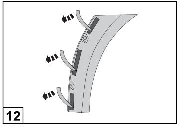
On the inside of the bumper flare remove approximately 25mm of the protective liner from the double sided tape locations. Fold the liner over and secure with masking tape to the outside of the fender flare.
