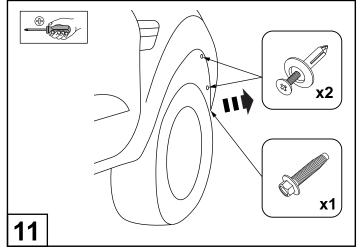
Remove and retain (2) scrivets from the wheel arch on the front bumper. Remove and retain the Hex head screw located under the bumper.
