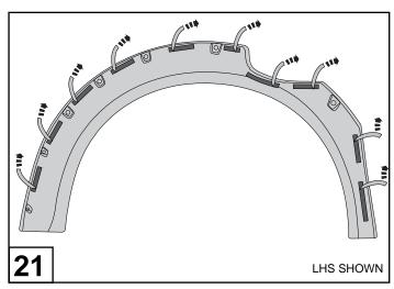
On the inside of the fender flare remove approximately 25mm of the protective liner from the double sided tape locations. Fold the liner over and secure with masking tape to the outside of the bumper flare.
