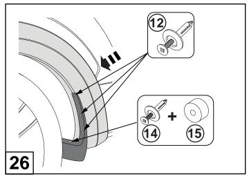
Fit the Mud Flap to the Fender Flare and secure with (3) 6mm plastic scrivets and one 10mm scrivet at the bottom, with one 5mm spacer.
