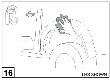
Wash the areas of contact on the vehicle and wipe dry. Wipe the fender where the flare will contact, using provided Alcohol wipes.
