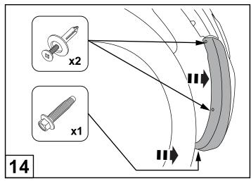
Secure the flare using previously removed scrivets and screw as shown.
