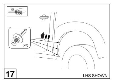
Remove the (3) scrivets from inside the rear wheel arch as shown.
