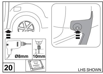
Carefully drill through centre of rivet holding the liner with a Ø8mm drill bit & and 10mm drill stop as shown. Carefully remove the reminder of the rivet using needle nose pliers. Apply rust inhibitor to the holes.
