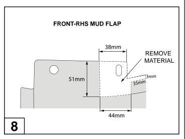
Measure and mark Mud Flap area to be removed, as shown. Using tin snips remove the white area. Repeat for the LHS Mud Flap. Remove all the masking tape.
