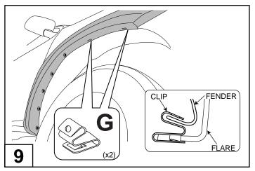
Install the clip at an angle, by pushing it on to the fender lip and then rotate downwards.
