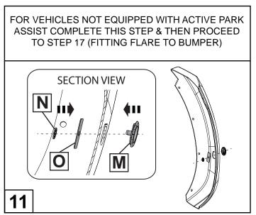
Fit the sensor cap and retaining strap to the fender flare, and secure with the starlock washer.
