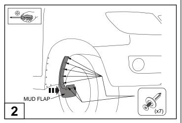
Remove the mud flaps by removing and retaining the (7) scrivets from inside the wheel arch as shown. NOTE: Replacement scrivets are supplied, if any scrivets are damaged upon removing from the vehicle.
