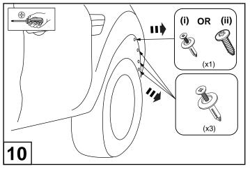
Remove all fixing, either (i) (scrivets x4) or (ii) (screw x1 and scrivets x3) from the wheel arch on the front bumper.
