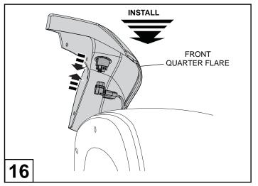
Hold fender flare assembly close to the bumper & fit Active park assist sensor to the escutcheon as per the Ford Workshop Manual (note the audible 'click' when the sensor is fully home).
