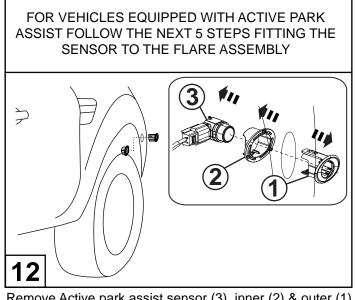
Remove Active park assist sensor (3), inner (2) & outer (1) escutcheon from bumper as per the Ford Workshop Manual.
