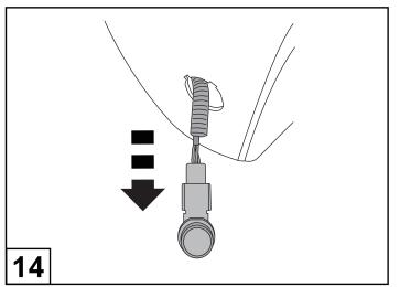
Pull extra harness length gently through the OEM hole in the bumper & refit in the Active park assist sensor; leave loosely ready to fit to the fender flare.
