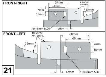
Measure & mark slot position & Mud Flap area to be removed, as shown. Using tin snips remove the light grey area. Cut 6x18mm slot using a die grinder. Remove all the masking tape.
