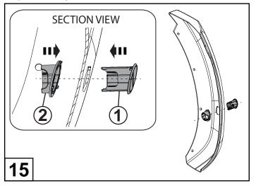
Fit inner (2) & outer (1) escutcheon for the Active park assist sensor to the fender flare assembly.
