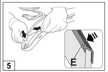
Pulling at right angles to the extrusion, remove the liner from the extrusion in small portions and apply thumb pressure to ensure that it adheres to the Fender Flares. Trim any unnecessary extrusion and discard.
