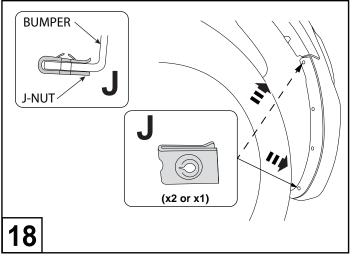
Hold the splash guard inwards and either (i) (push J-nut x2 in the top and bottom hole) or (ii) (if vehicle nutsert already exist in top hole, push J-nut in the bottom hole) as shown.
