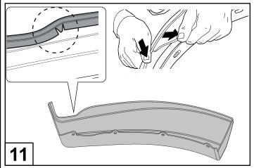
Pulling at right angles to the extrusion, remove the liner from the extrusion in small portions and apply thumb pressure to ensure that it adheres to the Fender Flares. Cut few triangle relief cuts in the extrusion (on the inside edge) to help the Fender Flare Extrusion conform to the shape of the flare as shown.
