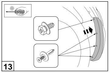
Secure the fender flare to the wheel arch with 3 scrivets and 1 screw as shown.
