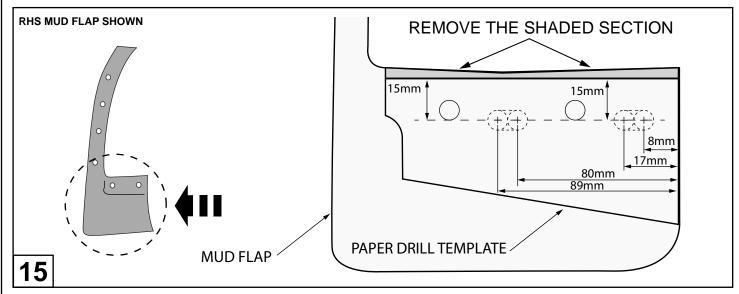
Print 1:1 scale paper drill template on the last page. Cut it out and stick to the back of the front mud flap using the 2 existing holes to position the template. Trim the top edge of the mud flap as shown, using tin snips. Mark the 4 slot centres as shown from the inside edge and drill with 8mm drill. Join two holes to create slot using die grinder or drill. Repeat the same on the LHS mud flap.
