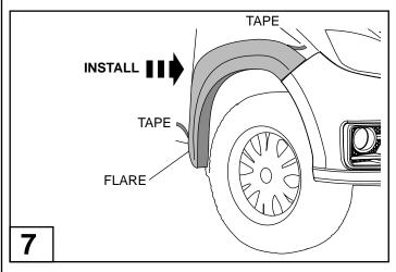
Peel back red tape liner, about 50mm from each corner of the adhesive tape on the back of the fender flare extrusion. Fit the flare to the vehicle as shown.
