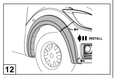
Peel back red tape liner, about 50mm from each corner of the adhesive tape on the back of the fender flare. Fit the front quarter flare to the vehicle as shown
