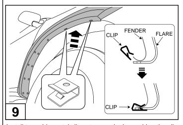
Install two wide metal clips at an angle, by pushing the clip on to the fender lip and then rotate downwards, as shown.
