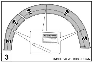
Using alcohol wipe clean the inside edge of each fender flare where the extrusion will adhere. Apply primer stick to the inside edge where the extrusion will adhere. Allow 3min for the primer to dry.
