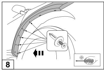
Install 5 wheel arch scrivets onto the flare as shown. While pressing and holding the flare in position of best fit.
