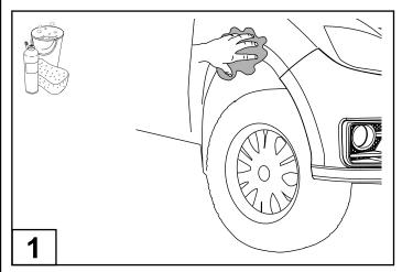
Wash the areas of contact on the vehicle and wipe dry both the vehicle and the Fender Flares with a clean cloth. Ensure inside of Fender Flares where extrusion will be attached is clean.
