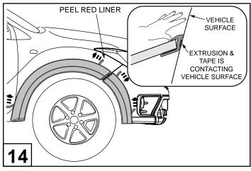
Ensure that flares are aligned. Remove the tape liner. Using your thumb and/or fingers apply firm pressure on the extrusion to ensure the extrusion and the tape is contacting the vehicle surface around the full perimeter of the flares.
