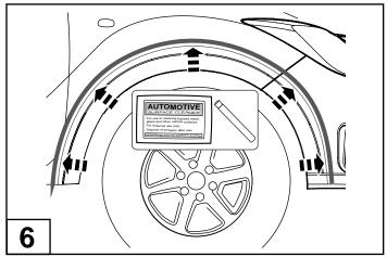
Using alcohol wipe clean the fender just below the tape, where the extrusion will adhere. Apply primer stick to the cleaned surface up to 10mm below the tape. Allow 3min for the primer to dry. Remove the tape.
