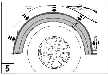
Test fit the fender flares to the vehicle and while holding the flares, apply masking tape to the fender just above the flares top edge. Remove the flares.
