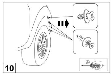
Remove 3 scrivets and 1 screw from the wheel arch on the front bumper.
