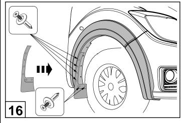
Secure the mud flap to the fender flare with 6 scrivets as shown.
