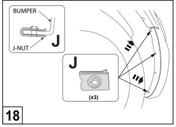
Hold the splash guard inwards and either (i) (push J-nut x3 in the top and bottom hole) or (ii) (if vehicle nutsert already exist in top hole, push J-nut in the bottom hole) as shown.
