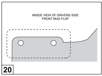
Prepare the Front Mud Flap by cleaning them & covering the marked areas with masking tape. Repeat for passenger side Front Mud Flap.
