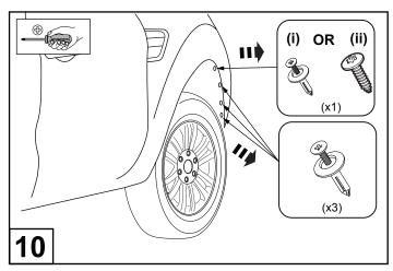
Remove all fixing, either (i) (scrivets x4) or (ii) (screw x1 and scrivets x3) from the wheel arch on the front bumper.
