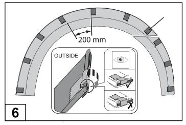
Apply masking tape as shown at 200mm intervals or where required to the fender flare extrusion. Fix the tape to the rear of the extrusion over the tape lining and over the front face of the Fender Flare. Ensure the tape does not overlap the tape lining and is not fixed to the inside surface of the fender flare.
