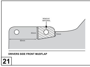
Measure & mark the dimensions as per the image on the mudflap. Using tin snips remove the light grey area. Once trimming is done, remove all the masking tape. Repeat for passenger side Front Mud Flap.
