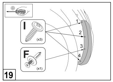
Hold the fender flare in the correct position ensuring the trim matches the bumper. Install the fixings as per the order in the image above.
