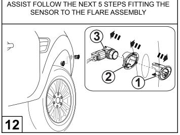
Remove Active park assist sensor (3), inner (2) & outer (1) escutcheon from bumper as per the Ford Workshop Manual.
