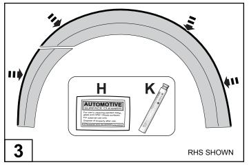
Clean the inside edge of each fender flare where the rubber extrusion will adhere with the Alcohol wipe and prime with the Primer Stick supplied.
