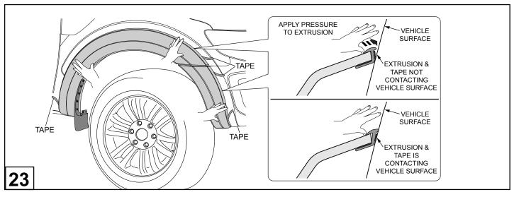
Ensure that flares are aligned. Remove the tape liner. Using your thumb and/or fingers apply firm pressure on the extrusion to ensure the extrusion and the tape is contacting the vehicle surface around the full perimeter of the flares.
