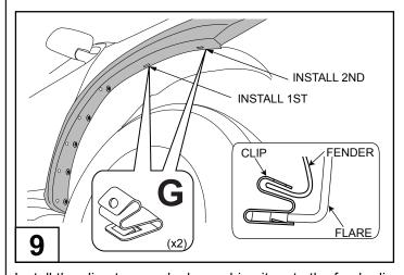
Install the clip at an angle, by pushing it on to the fender lip and then rotate downwards. Install the rear clip first and then install the front clip as shown on the picture.
