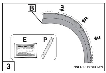
Clean the inside edge of the Rear Fender Flare (B) where the rubber extrusion will adhere with the Alcohol Wipe (E) and prime with the Primer Stick (P) supplied.
