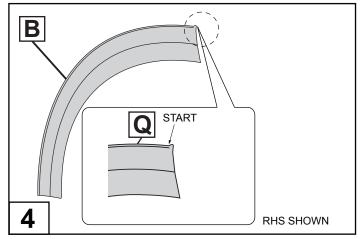
Remove approximately 50mm of the protective liner from the extrusion. Fit the extrusion (Q) to only the rear Fender Flare (B) along with the edge that comes in contact with the vehicle's body panel. **NOTE:** Start applying the extrusion from area shown above.
