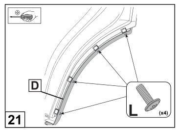
Ensure all holes with the flare and clips align. Adjust if required. Screw (L) the 4 M4x10 to secure.
