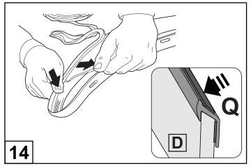
Pulling at right angles to the extrusion (Q), remove the liner from the extrusion in small portions and apply thumb pressure to ensure that it adheres to the Fender Flares. Trim any unnecessary extrusion and discard.
