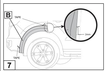
Mark 2mm from the edge of the split on the fender. Peel back red tape liner, about 50mm from each corner of the adhesive tape on the back of the fender flare (B). Now fit the flare to the vehicle on the marked spot 2mm away from the edge. **NOTE:** Ensure the Fender Flare is fitted as per the recommended 2mm from edge to prevent the rear flares looking spaced too far apart.
