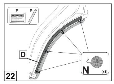
Wipe the inner side of the door with alcohol wipe and primer and use felt tape (N) provided to cover the fixings on the inner side of the door .
