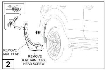
Remove the mud flaps by removing and retaining the (6) scrivets from inside the wheel arch and one Torx head screw as shown.
