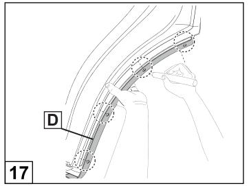
From the inside of the rear door hold the flare (D) in the position marked previously. Mark the position of the 4 holes in the flare against the inner door using a non permanent marker.
