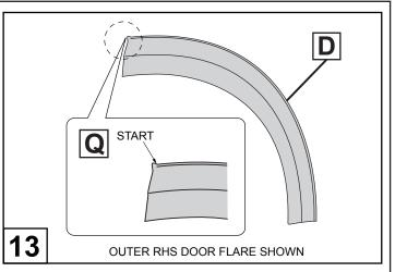
Remove approximately 50mm of the protective liner from the extrusion. Fit the extrusion to the Door Fender Flare (D) along with the edge that comes in contact with the vehicle's door. **NOTE:** Start applying the extrusion from area shown above.
