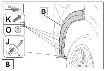
Install the 4 screws (K) and 4 Washers (O) where shown. Install the 1 Long Scrivet (J) where shown. Make sure the hardware is installed into the inner holes on the Fender Flare (B).
