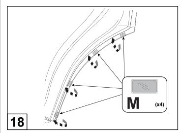
Stick the Anti Abrasive Tapes (M) over the door edge. Make sure the tapes are placed over the marked sections. Ensure both sides of the door are covered. (Tape folds over edge.)
