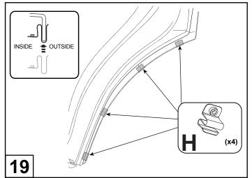
Push the 4 Clips (H). Over the Anti Abrasive Tapes. If the clip is loose on any of the locations, add an additional abrasive tape on top of the previous tape. **NOTE:** Ensure the center hole on each clip aligns with the 4 marks from step 12.
