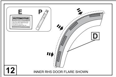
Clean the inside edge of the Fender flare (D) where the rubber extrusion will adhere with the Alcohol Wipe (E) and prime with the Primer Stick (P) supplied.
