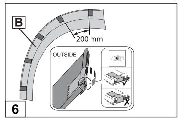
Apply masking tape as shown at 200mm intervals or where required to the fender flare extrusion (Q). Fix the tape to the rear of the extrusion (Q) over the tape lining and over the front face of the Fender Flare (B). Ensure the tape does not overlap the tape lining and is not fixed to the inside surface of the fender flare (B).
