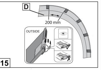
Apply masking tape as shown at 200mm intervals or where required to the fender flare extrusion (Q). Fix the tape to the rear of the extrusion (Q) over the tape lining and over the front face of the Fender Flare (D). Ensure the tape does not overlap the tape lining and is not fixed to the inside surface of the fender flare (D).
