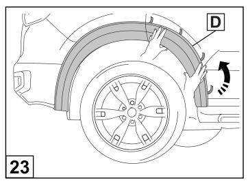
Remove the tape liners by pulling up and out. Discard of the liners. Ensure you remove them front to back. Apply pressure to the Flare (D) to ensure tape is fully seated to ensure maximum adhesion.
