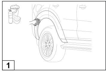
Wash the areas of contact on the vehicle and wipe dry both the vehicle and the Fender Flares with a clean cloth. Ensure inside of Fender Flares where extrusion is attached is clean.
