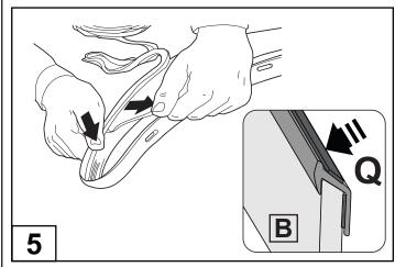
Pulling at right angles to the extrusion (Q), remove the liner from the extrusion in small portions and apply thumb pressure to ensure that it adheres to the Fender Flare (B). Trim any unnecessary extrusion and discard.
