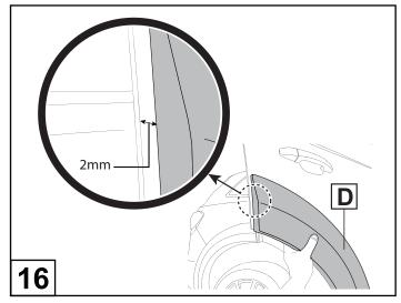
Position Fender Flare (D) against the door. Measure from the edge of the door to the Fender Flare as shown above, Ensure the Fender Flare is spaced 2mm away from the edge of the door. Mark the final position. **NOTE:** Ensure the flare is fitted as per the recommended 2mm from edge to prevent the rear flares looking spaced too far apart.
