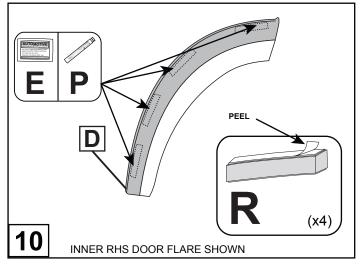
Use alcohol wipes (E) to clean the shaded areas, then apply primer stick (P) to the shaded area on the Door Rear Fender Flare (D). Peel away a small portion of tape liner on the tapered side of each Wedge Block (R) in preparation for fitting. **NOTE:** Do not apply Wedge Blocks in this step.
