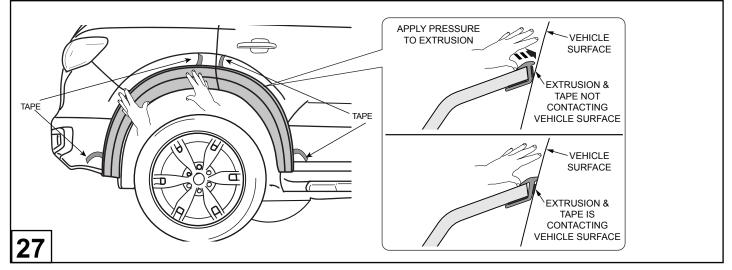
Ensure that flare is aligned. Remove the tape liner. Using your thumb and/or fingers apply firm pressure on the extrusion to ensure the extrusion and the tape is contacting the vehicle surface around the full perimeter of the flares.
