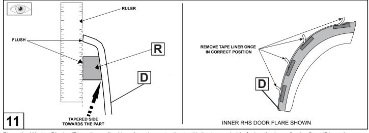
Place the Wedge Blocks (R) on the scribed locations (one at a time) with the tapered side facing the inner fender flare (D) as shown above. Check that the Wedge Block (R) is flush with the edge of the fender flare (D) using a ruler. If the Wedge Block (R) and fender flare (D) are not flush, move the Wedge Block (R) slightly downwards until both components sit flush. Once the position is confirmed, peel back the remaining tape liner to fix in position. This step applies to all 4 Wedge Blocks (R).
