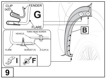
Ensure the Fender Flare (B) is still in position 2mm from away from the edge. Install clip (G) (x2) by pushing it on to the fender flip and then rotate downward in the order shown. Using scrivet (F) attach the Z-clip (I) to the fender flare into the hole on the underside. Secure the Z-clip to the vehicle using the retained Torx head screw from mudlfap.
