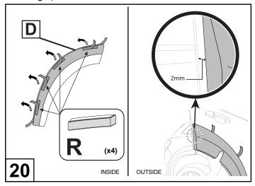
Peel back approximately 20mm of Tape liner from the Wedge Blocks (R). Also peel back about 50mm from each corner of the adhesive tape (red tape liner) on the back of the fender flare (D). Fit Flare (D) to the rear door. Make sure the 2mm gap from flare to door edge is present.
