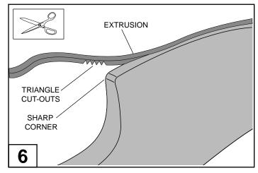
To fit the extrusion around sharp corners, cut a multiple triangles out of the extrusion where it meets the sharp corners as shown.
