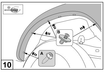
Secure the Fender Flare with (2) previously removed screw (A) and (3) plactic scrivets (B).
