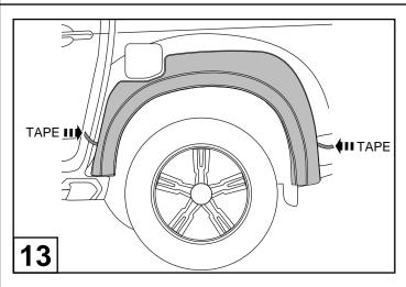
Remove the tape liner. Apply firm pressure on the flare to ensure the tape is contacting the vehicle surface around the full perimeter of the flares.
