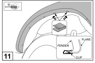
Fit (2) narrow clip as shown, ensuring the notch in the clip locates securely into the slot in the Fender Flare.
