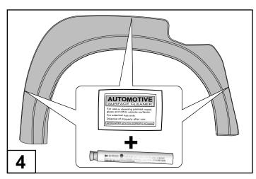
Where the rubber extrusion will adhere, clean the inside edge of each fender flare with alcohol wipe and apply primer.
