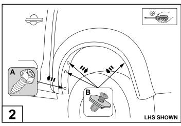
Remove and retain (3) plastic scrivets (B) from the wheel arch. Remove and retain (1) screw (A) from the fender.
