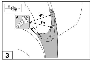
Remove the mud flaps by removing and retaining the (3) screws (A) from inside the wheel arch as shown.
