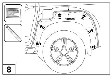
Remove the flare and use alcohol wipes to clean 10mm of the area inside side from the tape and apply a prime stick.
