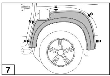
Place and hold the flare against the car and get a second person to mask the border around the flare using masking tape. Remove the flare and use alcohol wipes to clean 10mm of the selected area and then apply a prime stick in the selected area.
