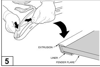
Remove approximately 50mm of the protective liner from the extrusion. Fit the extrusion to the Fender Flares along the edge that comes in contact with the vehicle's body panel. Trim any unnecessary extrusion and discard.
