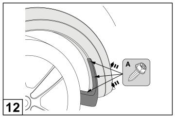
Fit the Mud Flap to the Fender Flare and secure with three (3) screws (A) as shown.
