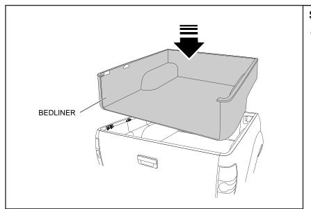
• Reinstall the tubliner, ensuring the alterations to the liner align neatly with the brackets on the tub.
