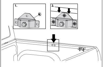
**Required tools:** Rivet gun, 13mm spanner and 13mm socket and driver.
