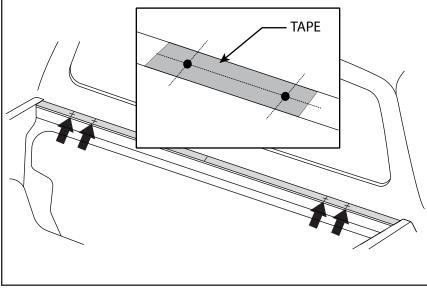
**Required tools:** Power drill, 8mm drill bit and drill bit stopper, centre punch, hammer.
