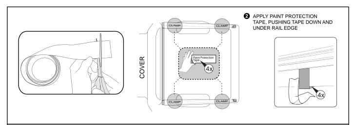
**8.** Cut out 4 sections (each of width 30mm) of Protection tape from the roll and apply it on the tub in the location marked 'CLAMP' on the side rail.
