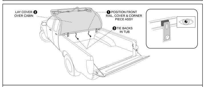
**4.** Position the front rail at the front of the tub. Carefully lay the cover over the vehicle cabin. Ensure Tie Backs are in the tub.
