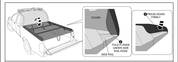
13. Roll cover over tub towards the rear of the vehicle. Fix the cover to the side rails by folding the flexible flanges on the cover outward and rolling them in under the edge of the side rails. To lock them in press firmly on the outside of the cover.
