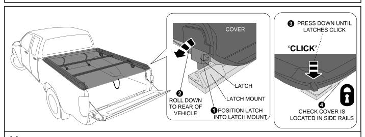
14. Position latches into stretch mounts. Holding the cover rail at the rear, roll towards the rear of the vehicle and down until latches click and are both locked into position. Ensure the flexible side flanges are fully seated into the side rails.
