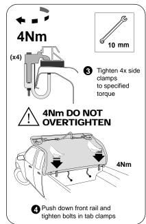
11. Centralise and align tonneau cover and rails. Check position of side rails by rolling tonneau cover out and ensuring that side latches engage into side rail end blocks on rear of tonneau cover. When correctly aligned lay cover back on vehicle roof and tighten both front and rear side clamps to the torque specified and push down front rail and tighten front tab bolts to the torque specified.
