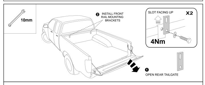
3. Install front rail mounting brackets into existing holes in front tub using M6 screws and washers provided.
