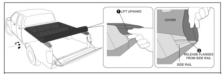
2. Working from the Rear to the Front of the Vehicle, Grip & Lift in an upward direction the Sides of the Cover to Release the Flexible Flanges from the Side rails.
