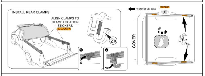
**10.** Repeat process and install Rear clamps the side rails and tub ensuring that the side rails are flush with the outside of the tub body.
