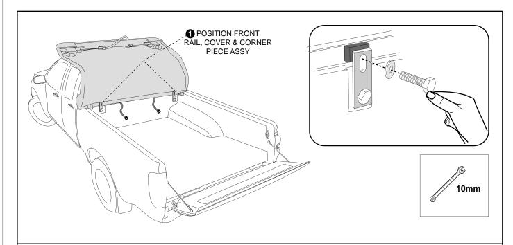
**5.** Align the threaded inserts in the Front Tonneau Cover Rail with the top holes of the Front Rail Tab Clamps and insert M6 Bolts and Washers and hand tighten.
