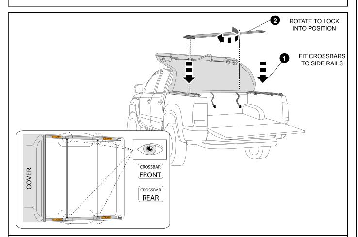
12. Fit the Cross Bar marked 'Front' closest to the Cabin & the Cross Bar marked 'Rear' closest to the Tailgate Note identification stickers on side rails showing positions.
