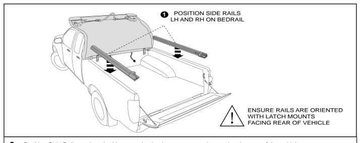
6. Position Side Rails on the tub sides ensuring latch mounts are orientated to the rear of the vehicle
