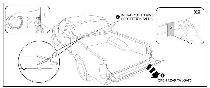
2. Cut out 2 sections (each of width 30mm) of Protection tape from the roll. Make a screw clearance hole in these 2 tapes. Align the hole in the tape with the hole in the tub as shown in the diagram above and apply the tape.
