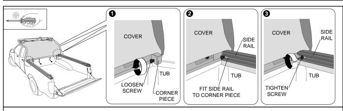
7. Loosen screws (ensuring they do not disengage from the backing nuts) on each side of the front rail corners. Engage the side rails into the front rail corner pieces ensuring they are fully seated. Tighten screws on both sides to firmly clamp the side rails to the front rail.
