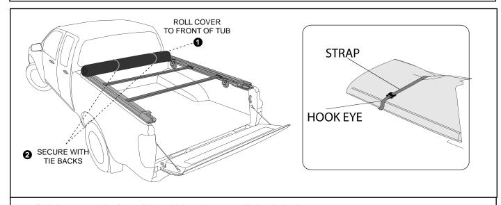
3. Roll the cover to the front of the vehicle and secure with the tie backs.
