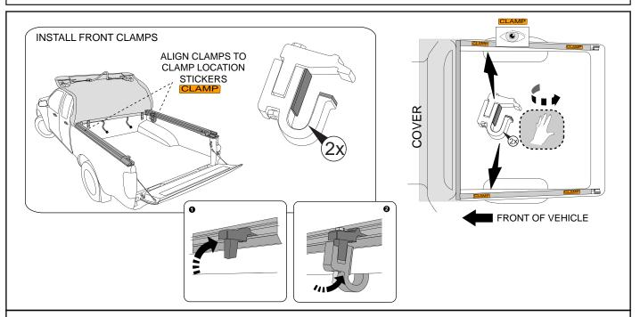
**9.** Using the clamp location stickers on the side rails, mount Front Clamps to the tub body ensuring that the side rails are flush with the outside of the tub body.
