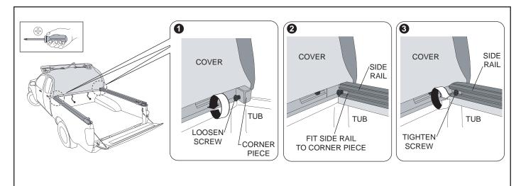
Loosen screws (ensuring they do not disengage from the backing nuts) on each side of the front rail corners. Engage the side rails into the front rail corner pieces ensuring they are fully seated. Tighten screws on both sides to firmly clamp the side rails to the front rail.
