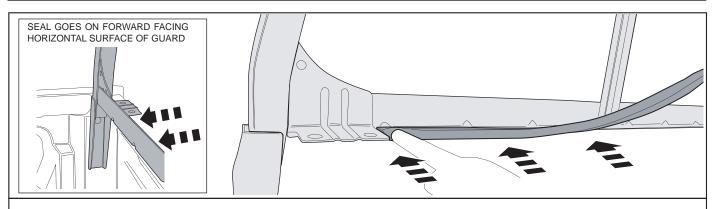
3. Install the cabin guard seal on to the cabin guard front area.
