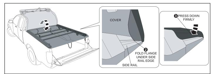
15. Roll cover over tub towards the rear of the vehicle. Fix the cover to the side rails by folding the flexible flanges on the cover outward and rolling them in under the edge of the side rails. To lock them in press firmly on the outside of the cover.
