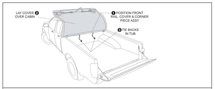
**6.** Position the front rail at the front of the tub. Carefully lay the cover over the vehicle cabin. Ensure Tie Backs are in the tub.
