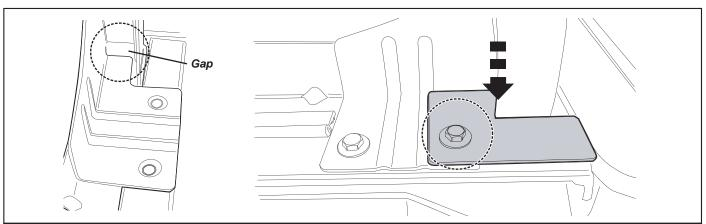
**5.** Place the front brackets in the corresponding pockets of the cabin guard. Align the brackets to close the gap and tighten them.
