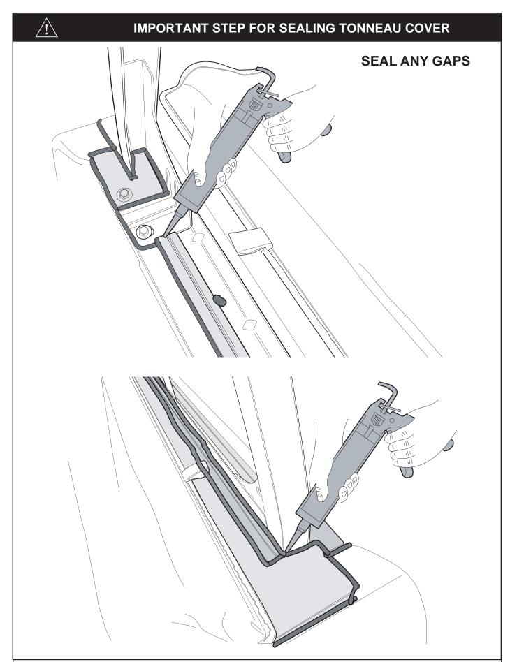
**18.** Seal all the gaps in and around cabin guard by applying Silicon gel (Not supplied). Allow the silicon gel to dry before any activity. This step is important, as it minimises leakage into the tray body in wet conditions.
