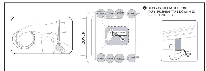
**9.** Cut out 8 sections (each of width 30mm) of Protection tape from the roll and apply it on the tub in the location marked 'CLAMP' on the side rail.
