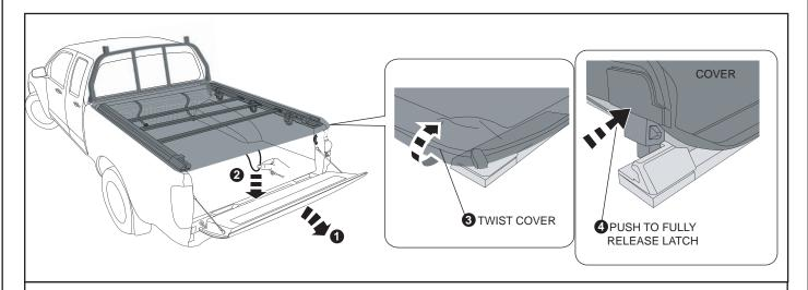
Open rear tailgate. Locate latch release tab under the centre rear of the cover and pull in a downward direction to disengage the latches. Twist the rear rail upward to completely release the latches.
