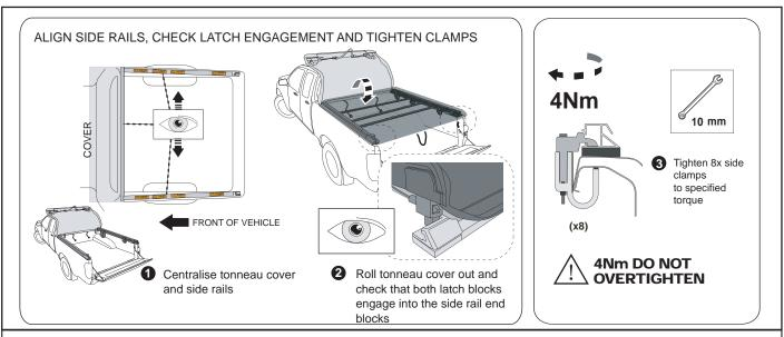
13. Centralise and align side rails. Check position of side rails by rolling Tonneau Cover out and ensuring that the side latches engage into side rail blocks on rear of Tonneau Cover. When correctly aligned lay cover back on the vehicle roof and tighten both front and rear side clamps to the torque specified.
