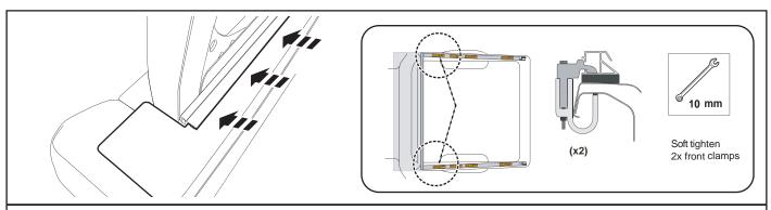
**12.** Push the SFTC Front plate / siderails forward against the cabinguard to close any gap between them. Soft tighten the Front clamps.
