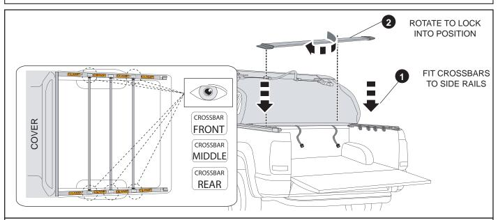
14. Fit the Cross Bar marked 'Front' closest to the Cabin & the Cross Bar marked 'Rear' closest to the Tailgate. Fit the Cross Bar marked 'Middle' in between the Front and Rear Cross Bars.
