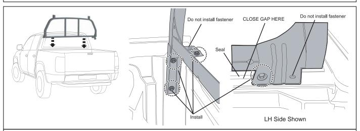
4. Install the cabin guard back on to the tub. (Ensure that the front gaps between the tub front board and the cabin guard are eliminated). NOTE: *Only install the screw on the inside of the cabinguard.*
