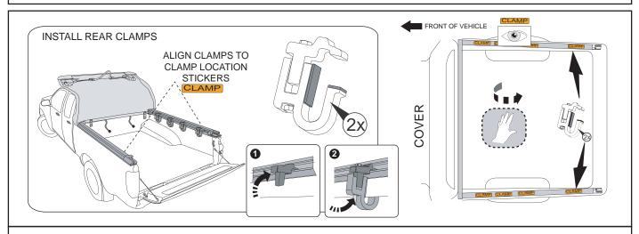
**11.** Repeat process and install Rear clamps the side rails and tub ensuring that the side rails are flush with the outside of the tub body.
