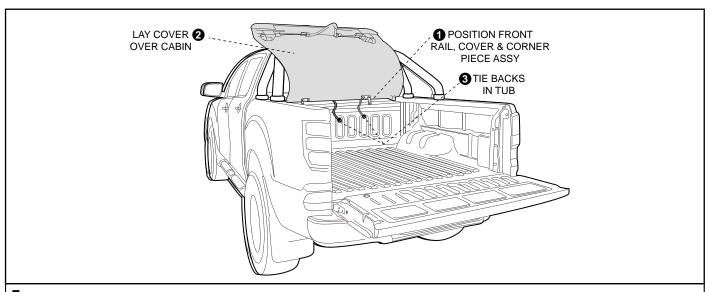
**5.** Position the front rail at the front of the tub. Carefully lay the cover over the vehicle cabin. Ensure tie backs are in the tub.
