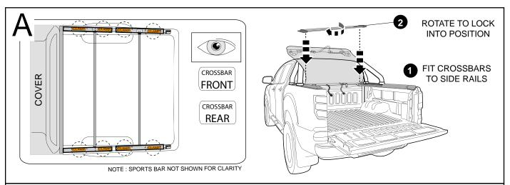
**13.** Fit the Cross Bar marked 'Front' closest to the Cabin & the Cross Bar marked 'Rear' closest to the Tailgate. Refer identification stickers on side rails showing positions.
