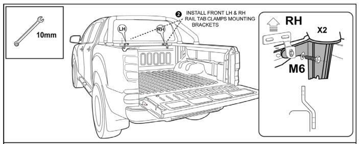
**4.** Install front rail tab clamps mounting brackets LH & RH into existing holes in sportsbar bracket / tub using M6 screws and washers provided. Do not tighten fully.
