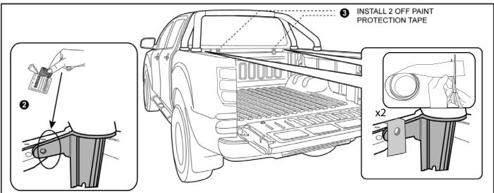
3. Cut out 2 sections (each of width 30 mm) of paint protection tape from the roll. Make a clearance hole in the 2 tapes. Clean the tub/ sportsbar bracket area with alchohol wipes, align the holes in the paint protection tape with holes in the sportsbar bracket as shown in diagram above and apply tape.
