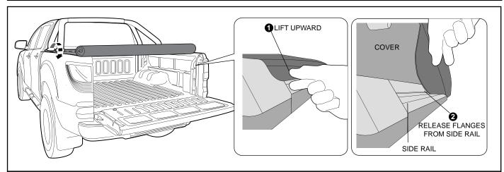
2. Working from the Rear to the Front of the Vehicle, Grip & Lift in an upward direction the Sides of the Cover to Release the Flexible Flanges from the Side rails.
