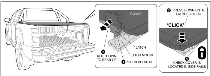
**16.** Position latches into stretch mounts. Holding the cover rail at the rear, roll towards the rear of the vehicle and down until latches click and are both locked into position. Ensure the flexible side flanges are fully seated into the side rails.
