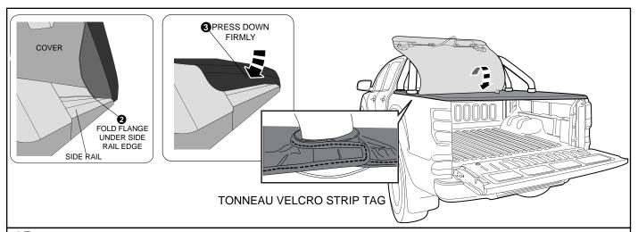
**15.** Roll cover over tub towards the rear of the vehicle. Fix the cover to the side rails by folding the flexible flanges on the cover outward and rolling them in under the edge of the side rails. To lock them in press firmly on the outside of the cover. Wrap the tonneau velcro strip tag around the sportsbar foot and seal it.
