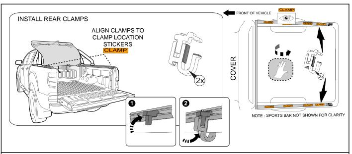
**11.** Repeat process and install Rear clamps the side rails and tub ensuring that the side rails are flush with the outside of the tub body.
