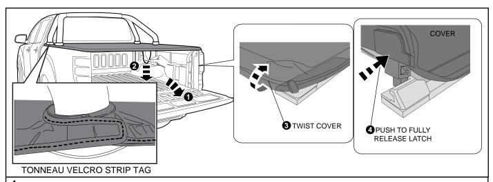
1. Open rear tailgate. Release the tonneau velcro strip tags from the Sports Bar foot.
