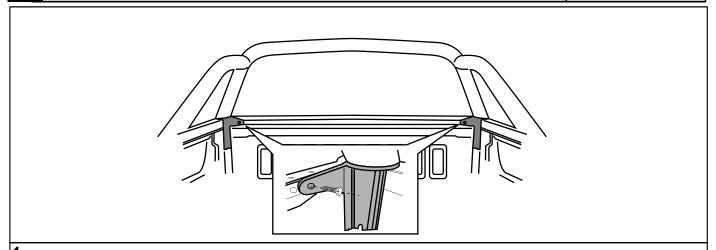
1. Remove the existing sportsbar bracket front screw (2 off). Note:Do not remove the sportsbar bracket screws on the sides.
