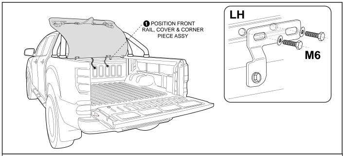
**6.** Align the threaded inserts in the front Soft Tonneau Cover Rail with the top holes of the Front Rail Tab Clamps and insert M6 Bolts and Washers and hand tighten.
