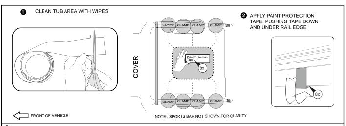
**9.** Clean the tub areas with alcohol wipes in the location marked 'CLAMP' on the side rails. Cut out 8 sections (each of width 30 mm) of Protection Tape from the roll and apply it on the tub in the location marked 'CLAMP' on side rail.
