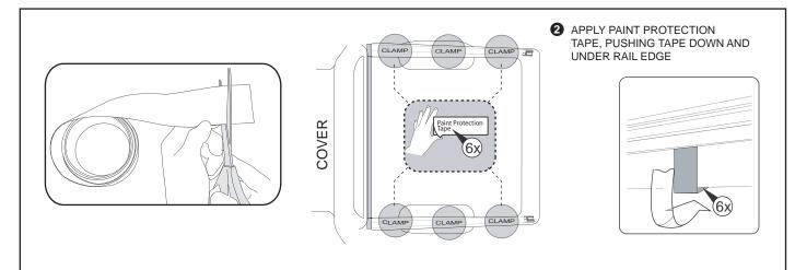
**9.** Cut out 4 sections (each of width 30mm) of Protection tape from the roll and apply it on the tub in the location marked 'CLAMP' on the side rail.
