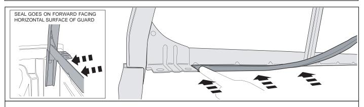
$\ensuremath{\mathbf{3}}\xspace$  . Install the cabin guard seal on to the cabin guard front area.
