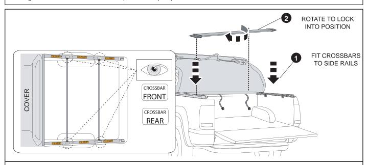
14. Fit the Cross Bar marked 'Front' closest to the Cabin & the Cross Bar marked 'Rear' closest to the Tailgate Note identification stickers on side rails showing positions.
