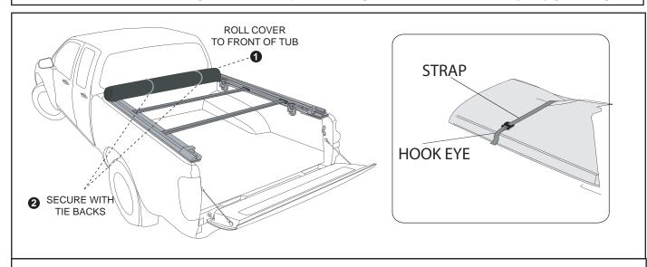
$\boldsymbol{3.}\,$  Roll the cover to the front of the vehicle and secure with the tie backs.
