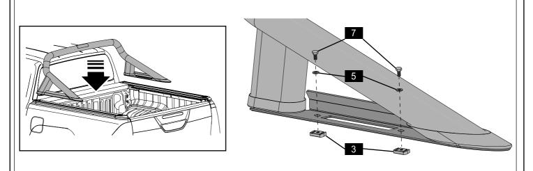
3. Carefully lower the sportsbar onto the side rails. Reposition the Slot Nuts (3) inside the T-channel to align with the holes in the Side Plates (1)(2). Loosely secure the RHS of the sportsbar in place with two M8 Hex Head Bolts (7) and two Large Washers (5). Repeat for LHS.
