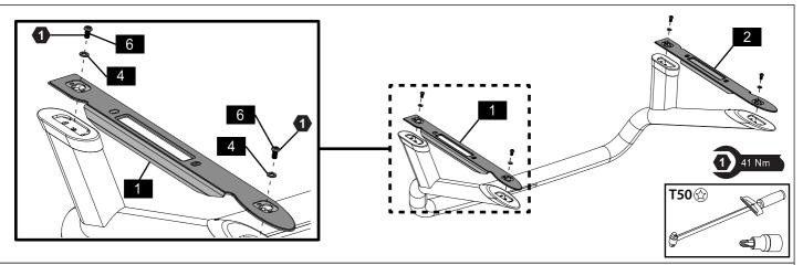
2. Carefully place the sportsbar upside down on a blanket. Secure the Right Side Plate (1) to the right feet of the sportsbar using two M10 Torx Screws (6) and two Small Washers (4), and tighten to 41Nm. Repeat for the LHS.
