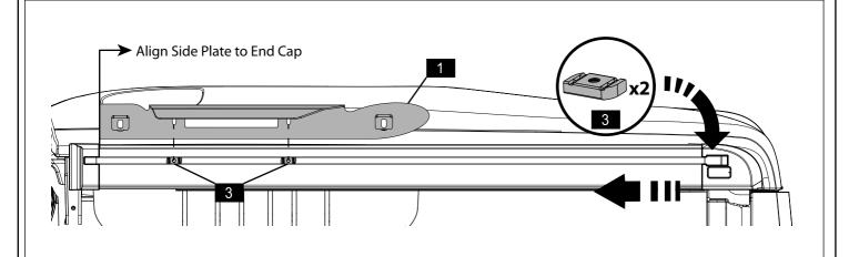
1. Slide two Slot Nuts (3) into the RHS T-channel of the side rail as shown. Position the RHS Side Plate (1) on the side rail, with the front edge of the Side Plate flush with the front end cap of the RollTrac. Ensure the Slot Nuts roughly align with the holes in the Side Plate. Repeat for LHS.
