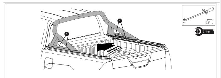
4. Slide the sportsbar back until both Side Plates (1)(2) are flush with the front end cap of the RollTrac. Tighten all M8 Hex Head Bolts (7) to 21Nm.
