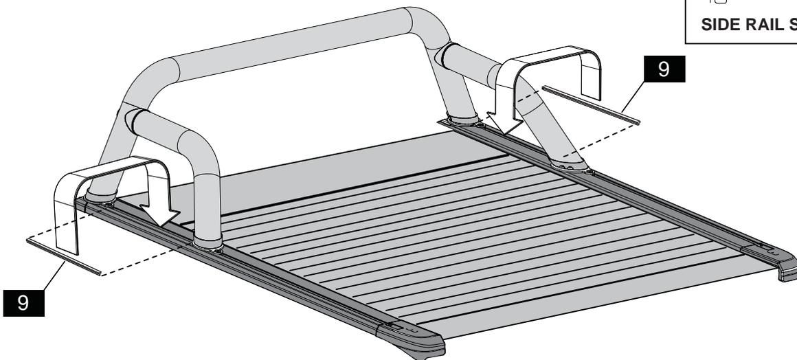
5. Measure the distance between the feet in the side rail channels and cut the T-Channel Extrusion (9) to length. Fit the T-Channel Extrusion into the side rail channels between the Sports Bar legs, by firmly pressing it into the channel recess.
