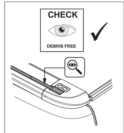
1. Prepare the surface of the side rails by cleaning them thoroughly ensuring that any debris in the side rail channels is completely removed.
