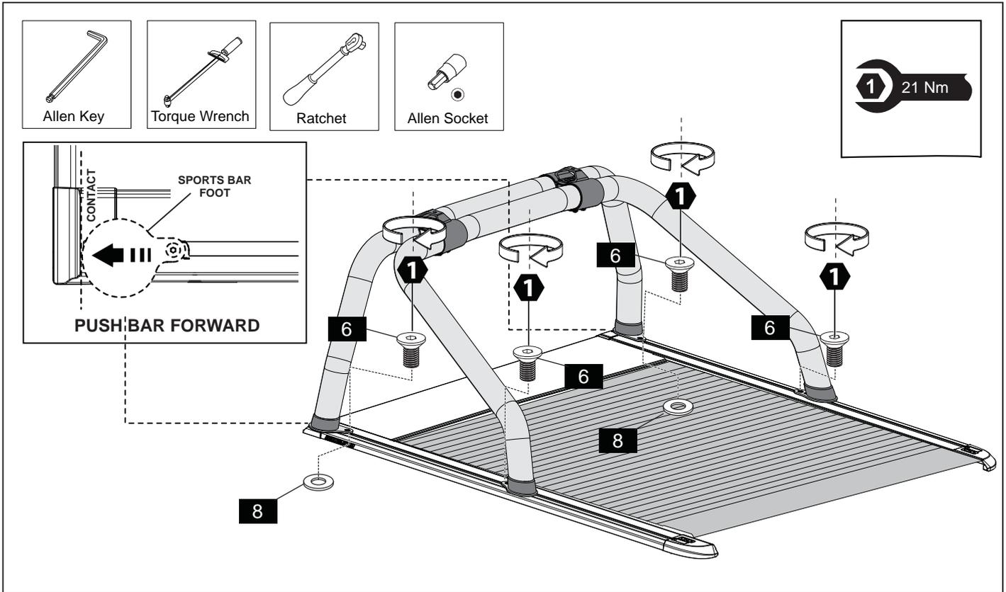
4. Push the sports bar forward so that the front feet are aligned with the front of the corner cap as shown. Reposition the M8 T Nuts (7) in the T-channel to align with the holes in the Foot Plates (1),(2),(3),(4). Place a washer (8) under front foot and then secure the sportsbar in place with four M8 Counter Sunk Socked Head Screws (6). Torque to 21Nm.
