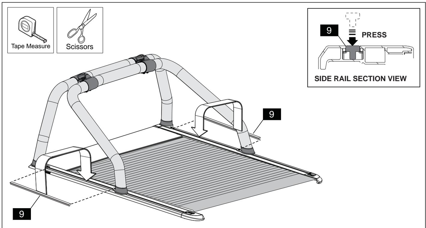
5. Measure the distance between the feet in the side rail channels and cut the T-Channel Extrusion (9) to length. Fit the T-Channel Extrusion into the side rail channels between the Sports Bar legs, by firmly pressing it into the channel recess.
