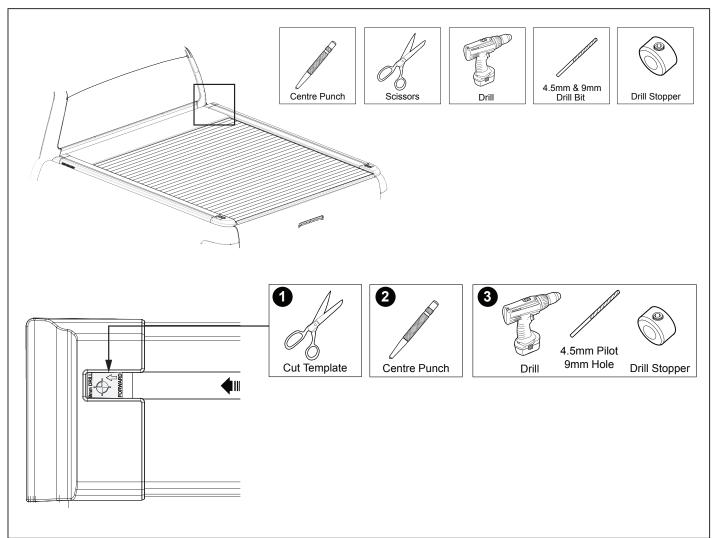
2. Cut out the template on Page 13, insert the template into the channel and push all the way to the end of the RHS Side Rail. Centre punch the hole location, pilot drill with a 4.5mm drill and then drill a 9.0 mm hole all the way through the side rail. Clean out any swarf from the channel and the tub.
