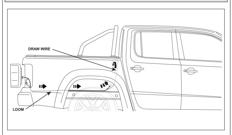
**18.** Route the Wiring Adaptor Loom (23) from the tail light compartment, behind the wheel arch towards the front right hand corner of the tub. Using the draw wire, pull the Wiring Adaptor Loom (23) up through the hole and into the Vehicle Tub.
