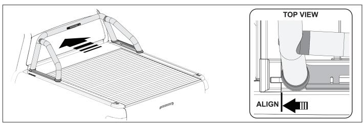
11. Position the Sports Bar such that the Mount Plates align to the RollTrac End Caps.
