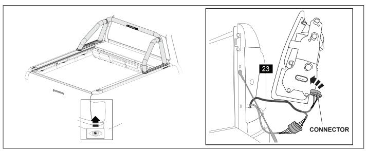
**17.** Bridge the male and female connectors from the Tail Lamp with the Wiring Adaptor Loom (23). Route the Wiring Adaptor Loom (23) under the tub.
