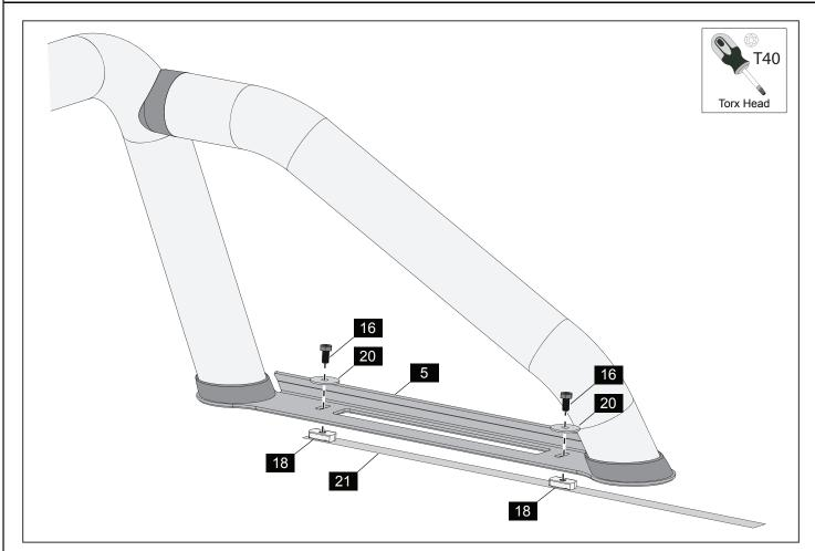
13. Reposition the Slot Nuts (18) inside the T-Channel using the Installation Aid (21) and align with the holes in the Mount Plate RHS (5). Loosely install the M8 Hex Head Bolts (16) and the Large Washers (20) through the Mount Plate RHS. Once both Screws are finger tightened, remove the Installation Aid from the T-Channel and repeat for the LHS.
