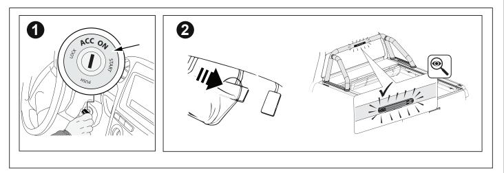
**23.** Power up accessories on vehicle, depress the brake pedal and check the function of the LED brake light on the Sports Bar.
