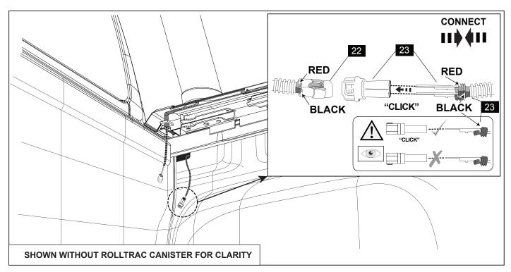
20. Attach the Loose Connector (23) to the Wiring Adaptor Loom (23)
