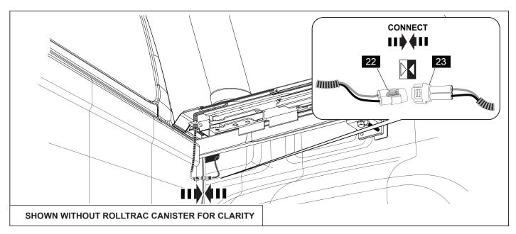
21. Attach the Loose Connector (23) to the Wiring Adaptor Loom (23).
