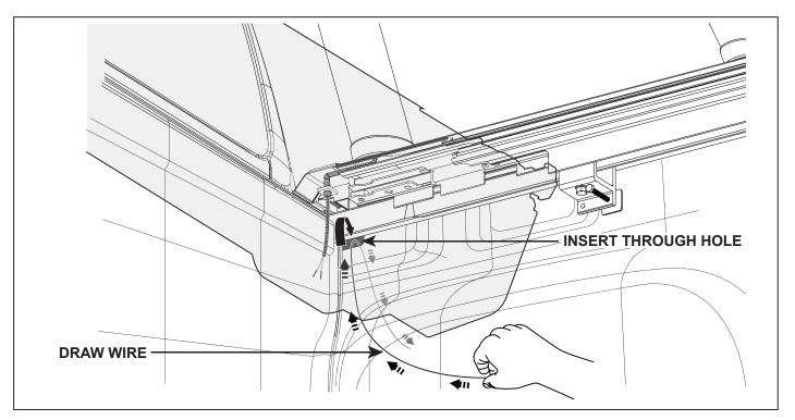
**15.** Insert a draw wire into the hole located at the front right hand corner of the tub. The hole is situated behind the Rolltrac housing.
