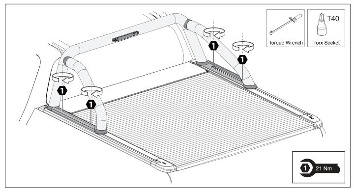
14. Tighten all M8 Hex Head Bolts (16) to 21Nm.
