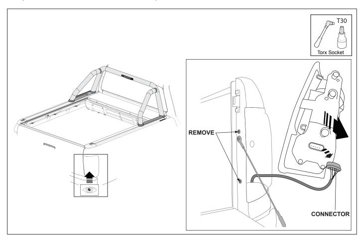
**16.**Remove the two bolts that secure the RHS Rear Tail Lamp. Disconnect the Tail Lamp Connector. Remove the RHS Tail Lamp.
