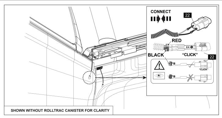
19. Attach the Electrical Plug (22) to the Stop Lamp wires as shown.
