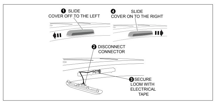
**9.** Remove the stop lamp plastic cover by sliding the cover from right to left. Disconnect the stop lamp electrical connectors as shown. Use electrical tape to protect each connector. Re-attach the stop lamp and stop lamp plastic cover.
