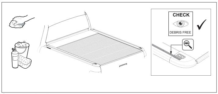
1. Prepare the surface of the side rails by cleaning them thoroughly ensuring that any debris in the side rail channels is completely removed.
