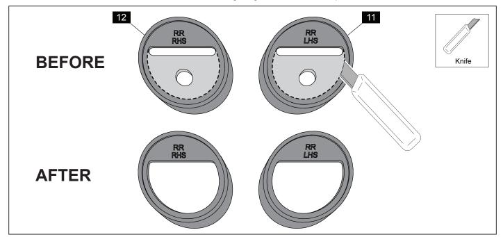
Locate the Foot Cups - RR LHS (11) and RR RHS (12).Mark then cut the Foot Cups as shown and discard the cut out sections (shown above).
