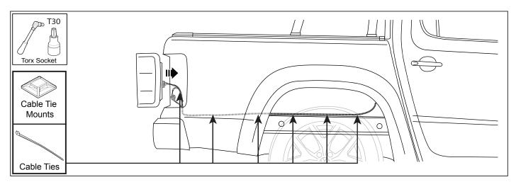
**22.** Secure the Wiring Adaptor Loom (23) to the vehicle at various points using the Cable Ties (24) and Cable Tie Mounts (25). Loop any excess wiring loom and secure with cable ties. Re-attach the RHS Tail Lamp.
