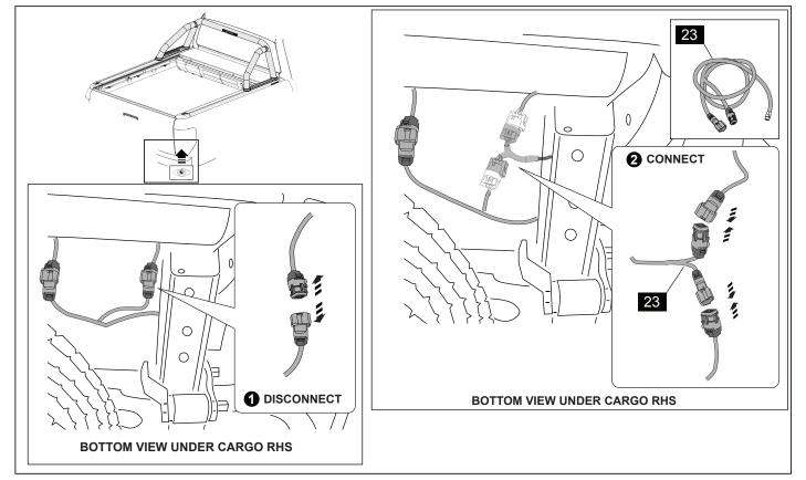
**16.** Locate the RHS Tail Lamp Connector underneath the Cargo RHS. Unplug the Tail Lamp Connector. Bridge the male and female connectors from the Tail Lamp with the Wiring Adaptor Loom (23).
