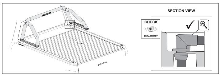
**10.** Position the sports bar above the tub and feed the sports bar loom through the hole in the RHS rail. Press the grommet into the hole in the side rail as shown ensuring that it is well seated. A trim removal tool can be used to seat the grommet.
