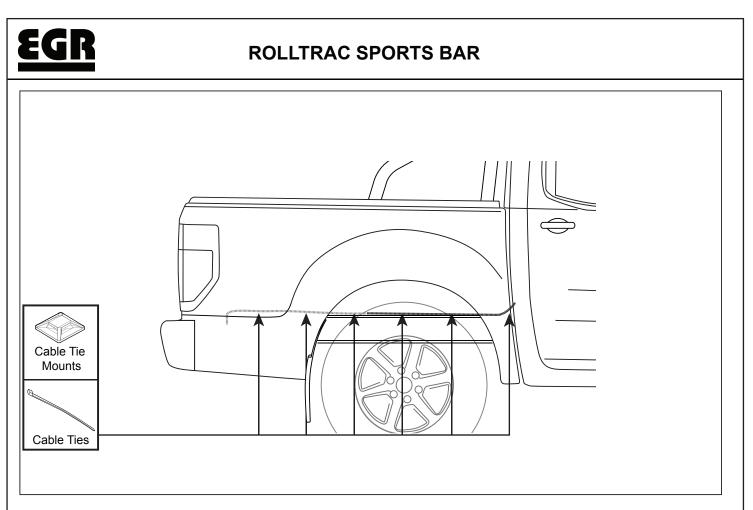
Secure the Wiring Adaptor Loom (23) to the vehicle at various points using the Cable Ties (24) and Cable Tie Mounts (25). Loop any excess wiring loom and secure with cable ties.
