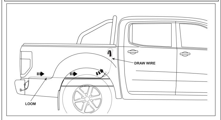
**17.** Route the Wiring Adaptor Loom (23) from the tail light compartment, behind the wheel arch towards the front right hand corner of the tub. Using the draw wire, pull the Wiring Adaptor Loom (23) up through the hole and into the Vehicle Tub.
