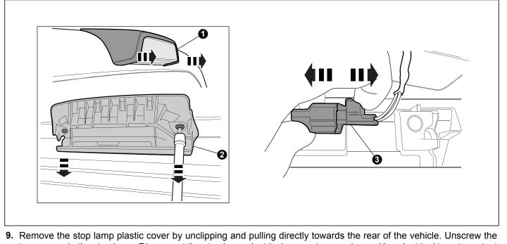
**9.** Remove the stop lamp plastic cover by unclipping and pulling directly towards the rear of the vehicle. Unscrew the two screws in the stop lamp. Disconnect the stop lamp electrical connectors as shown. Use electrical tape to protect each connector. Re-attach the stop lamp and stop lamp plastic cover.
