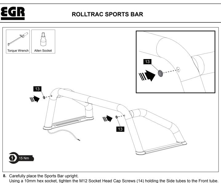
Using a 10mm hex socket, tighten the M12 Socket Head Cap Screws (14) holding the Side tubes to the Front tube. Torque to 15Nm.
