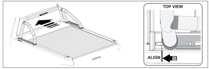
**11.** Position the Sports Bar such that the Mount Plates align to the RollTrac End Caps.
