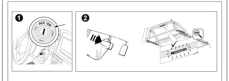
**22.**Power up accessories on vehicle, depress the brake pedal and check the function of the LED brake light on the Sports Bar.
