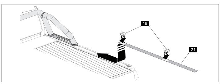
**12.** Insert the Installation Aid (21) into the T-Channel of the side rail. Slide two Slot Nuts (18) into the T-Channel and position them on top of the Installation Aid.
