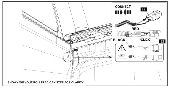
**18.** Attach the Electrical Plug (22) to the Stop Lamp wires as shown.
