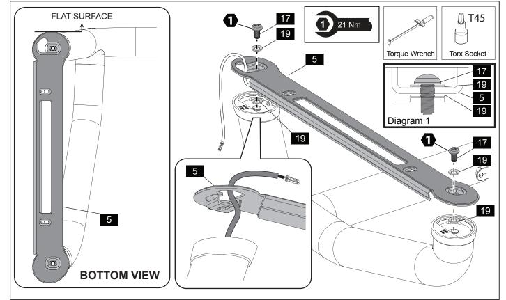
7. Place the Mount Plate RHS (5) onto the Sportsbar with the flat surface at the front of the Sportsbar. Feed the LED wiring loom through the front, side slot located on the Mount Plate RHS (5). Place a Small Washer (19) between the Mount Plate and Sportsbar foot at each screw position. Then secure the Mount Plate with M8 Torx Screw (17) and Small Washer (19). See Diagram 1 for detail. Tighten to 21Nm. Repeat for LHS.
