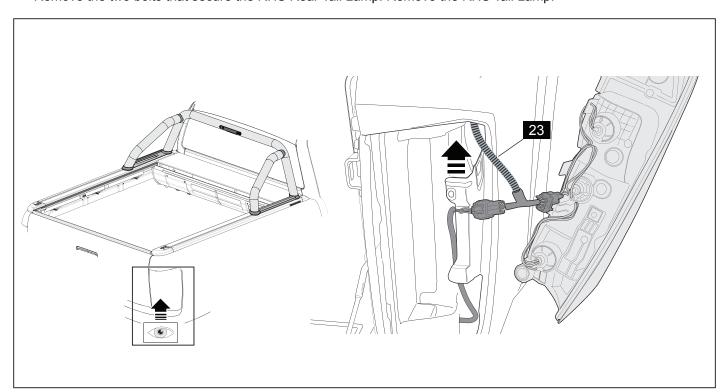
**18.** Unplug the tail lamp connector. Bridge the male and female connectors from the tail lamp with the Wiring Adaptor Loom (23). Route the Wiring Adaptor Loom (23) into the tail light compartment up through the opening at the top.
