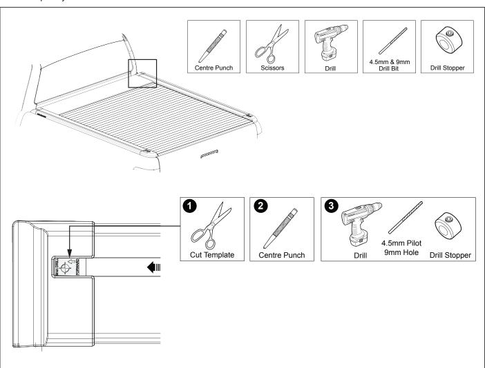
2. Cut out the template on Page 13, insert the template into the channel and push all the way to the end of the RHS Side Rail. Centre punch the hole location, pilot drill with a 4.5mm drill and then drill a 9.0 mm hole all the way through the side rail. Clean out any swarf from the channel and the tub.
