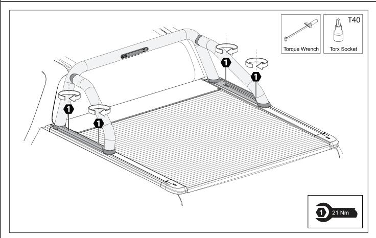
**13.** Tighten all M8 Hex Head Bolts (16) to 21Nm.
