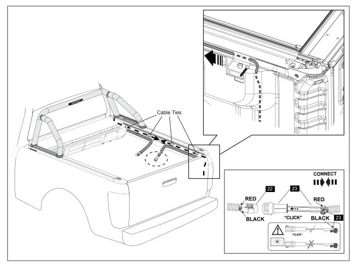
**19.**Route the Wiring Adaptor Loom (23) along the full length of the RollTrac. Attach the Loose Connector (23) to the Wiring Adaptor Loom (23) as shown.
