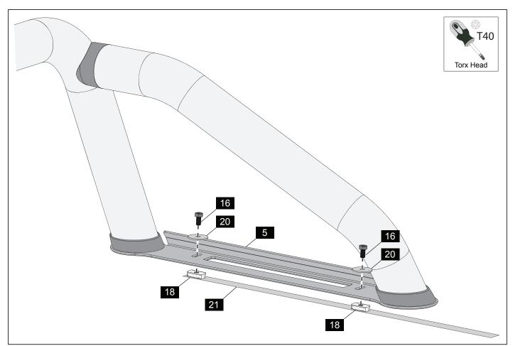
**12.** Reposition the Slot Nuts (18) inside the T-Channel using the Installation Aid (21) and align with the holes in the Mount Plate RHS (5). Loosely install the M8 Hex Head Bolts (16) and the Large Washers (20) through the Mount Plate RHS. Once both Screws are finger tightened, remove the Installation Aid from the T-Channel and repeat for the LHS.
