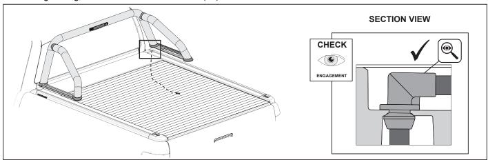
**9.** Position the sports bar above the tub and feed the sports bar loom through the hole in the RHS rail. Press the grommet into the hole in the side rail as shown ensuring that it is well seated. A trim removal tool can be used to seat the grommet.
