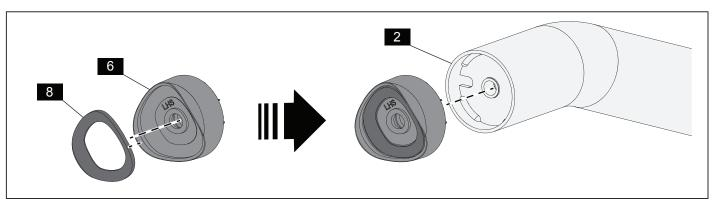
3. Install the Joiner LHS (6) to the top end of the Side Tube LHS (2). Ensure the locating pin on the joiner goes into the recess on the plate for alignment. Repeat for Joiner RHS (7) into the Side Tube RHS (3).
