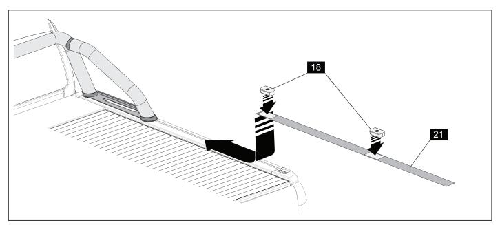
**11.** Insert the Installation Aid (21) into the T-Channel of the side rail. Slide two Slot Nuts (18) into the T-Channel and position them on top of the Installation Aid.
