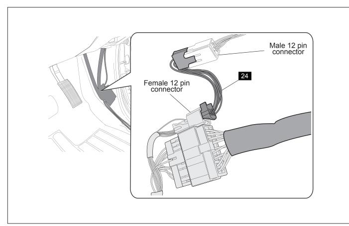
**15.** Locate the 12 Pin Connector as shown. Bridge the Male and Female connectors with the Connector Patch (24). Re-attach the retained Dash Trim Pad and Sill Plate.
