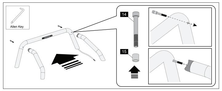
**4.** Add the Spacer (15) to each of the M12 Socket Head Cap Screws (14). Insert the Screw with Spacer through the front RHS hole of the Front Tube (1). Hold in place with a 10mm hex key. Install the Side Tube RHS to the Front Tube and finger tighten the screw. Repeat for LHS.
