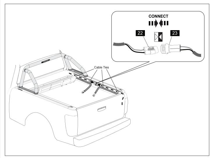
20. Connect the Wiring Adaptor Loom (23) to the Stop Lamp Wiring Loom (22). Secure the Wiring Loom to the Roll Trac at various points using the Cable Ties (25) and Cable Tie Mounts (26). Loop any excess Wiring Adaptor Loom (23) and secure with Cable Ties (25). Re-attach the RHS tail lamp.
