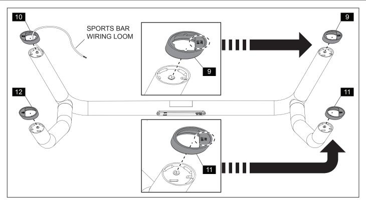
6. Carefully place the Sportsbar upside down. Push all four Foot Cups (9,10,11,12) onto the corresponding foot of the Sportsbar. When installing Foot Cup – FRT RHS (10), feed the Wiring Loom through the Footcup Hole before installing. Ensure the Foot Cups are correctly oriented, with text to the outside of the Sportsbar.
